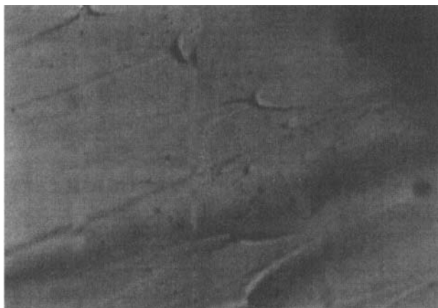
Fig.3. Microphotograph of a parabolic focal conic domains created in a planar sample of the SmA mixture 8CB/7AB by a He-Ne laser beam.
